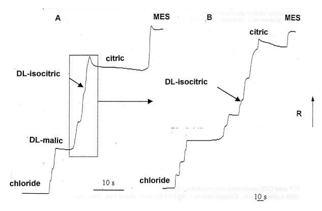
Fig. 1: ITP records of lime-juice sampleink. Sample was diluted 50-times.
